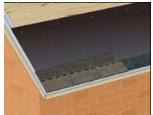
The sealant strip at the bottom edge allows for a tight seal at the bottom of the shingle.
